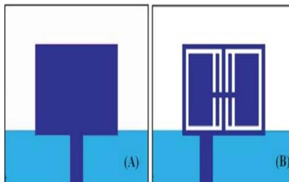
Figure 1. Evolution steps of antenna design
