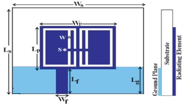
Figure 2. Antenna geometry and its side view.
